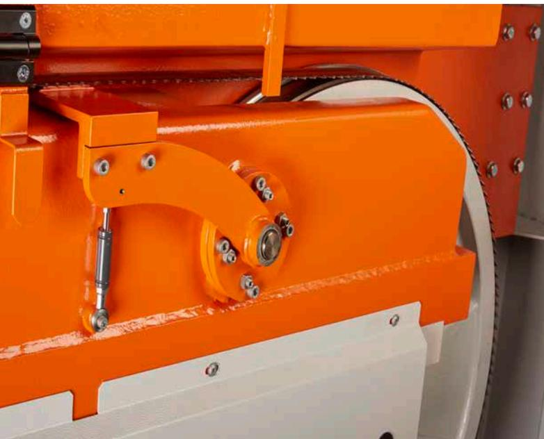
Modern machine tool construction: steel jacket cast with mineral casting
