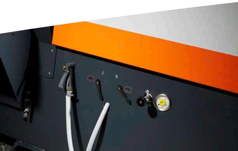
Coolant hose for cleaning the work area / clamping force regulation
