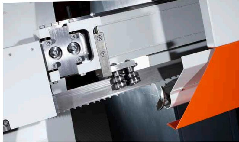
Rigid welding construction in horizontal position with pretensioned linear guides. Bandsaw blade guides with closed supply system. Integrated tool control sensors.
