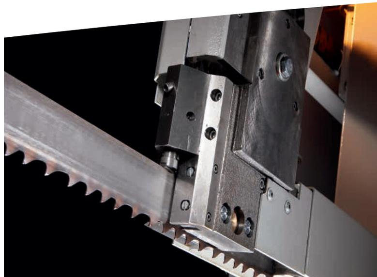
U-shaped tape guide head with band free lifting device.
