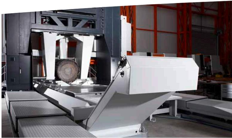
Chip conveyor with a conveying width of 1.250 mm and an ejection height of 1.100 mm
